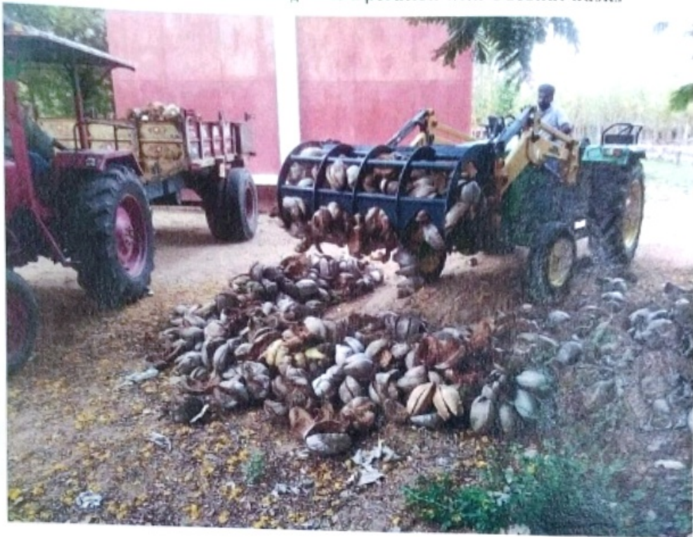
AGRIBULL – Grabbing fork Operation with Coconut husks
