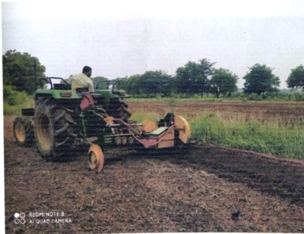
View of the ridge plaster/bund former during the field operation (dry land)
