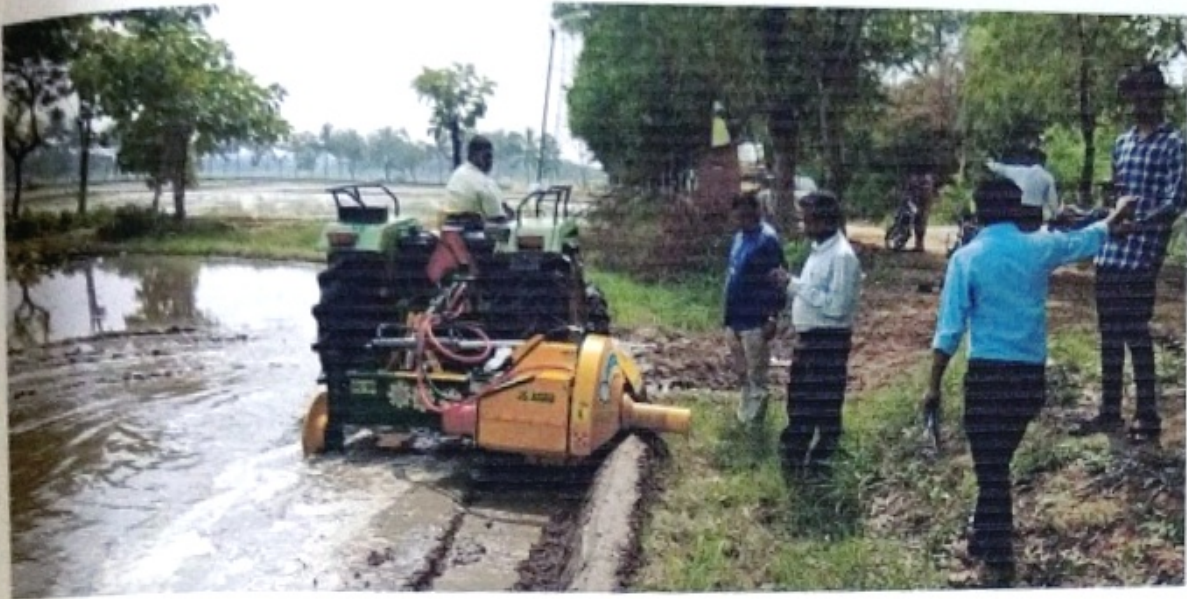
View of the ridge plaster/bund former during the field operation (Wet land)
