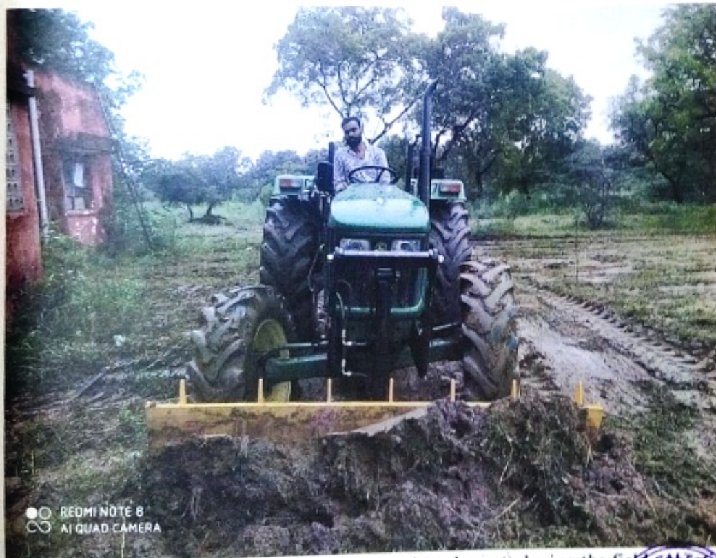
View of the bull front end dozer 6.5 feet (Tractor Attachment) during the field operation
