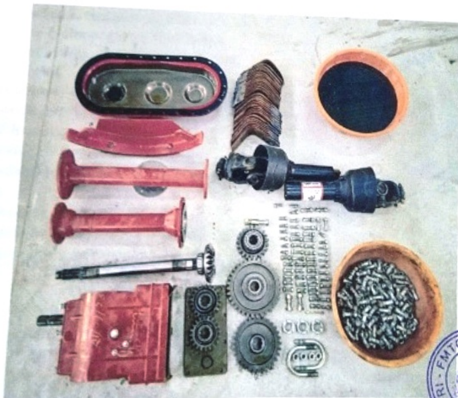
Fig. 8. Dismantled view of TAFE Agristar 512 VX rotavator gear box
