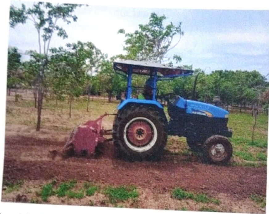
Fig.7 View of the TAFE Agristar 512VX rotavator during the field operation (Dry land)
