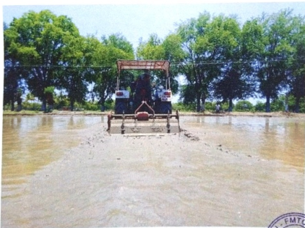
Fig.6 View of the TAFE Agristar 717 VX rotavator during the field operation (Wet land)
