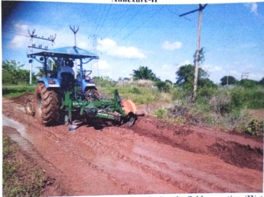
Fig 7. View of the ridge plaster/bund former during the field operation (Wet land)
