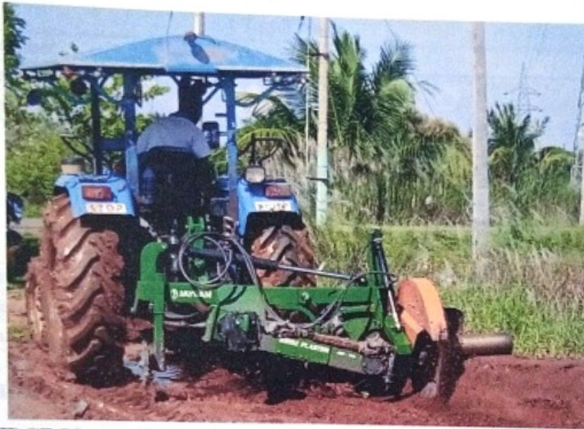
RIDGE PLASTER/ BUND FORMER (Dry & Wet) MODEL JRP-163 (TRACTOR MOUNTED)
