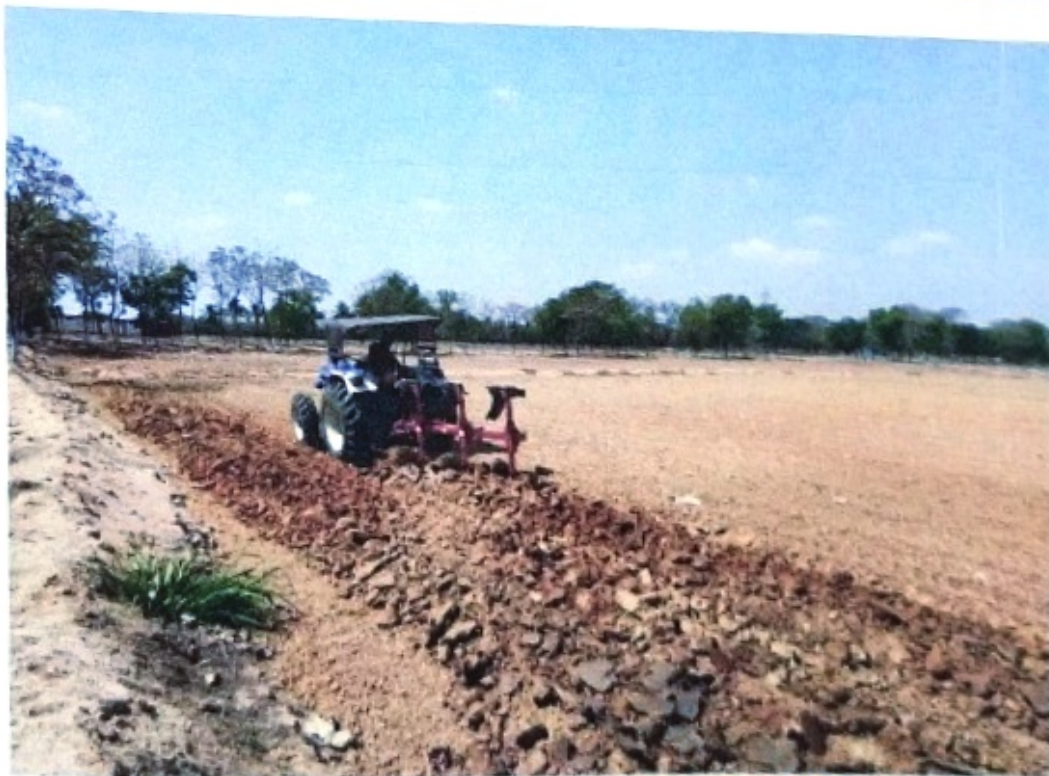
Fig.7. View of the Reversible Mould board plough during the field operation
