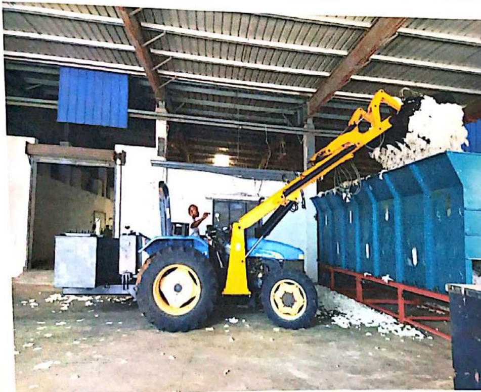
Fig. 6 Operational view of Log fork bucket
