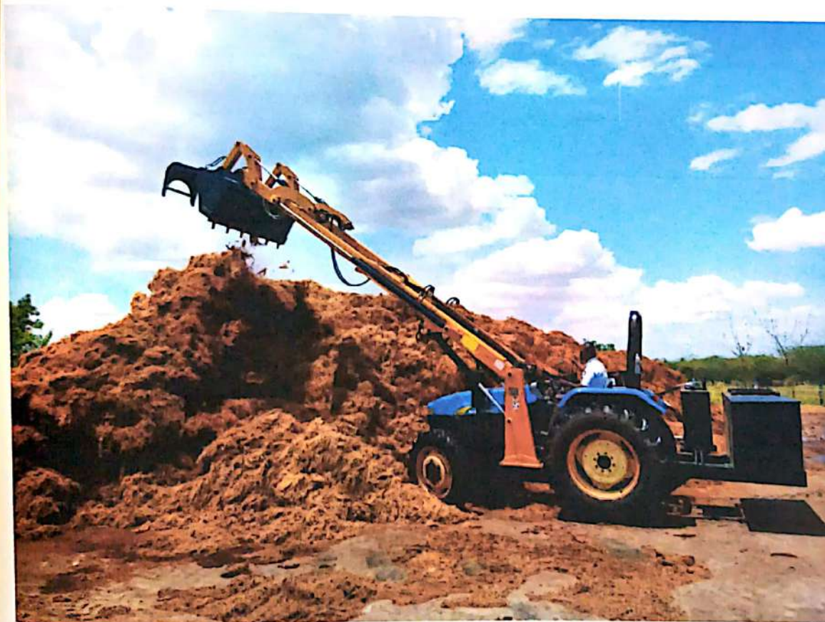
Fig. 5 Operational view of Grabbing Fork Bucket
