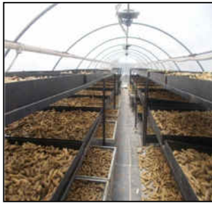
Turmeric dried in Hybrid Solar – Biomass dryer
