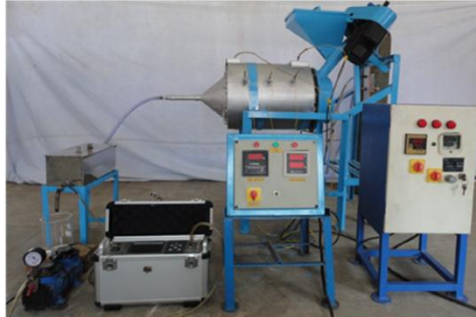
Developed pyrolytic reactor (1 kg/h)
