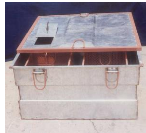
Improved farm level Turmeric boiler
