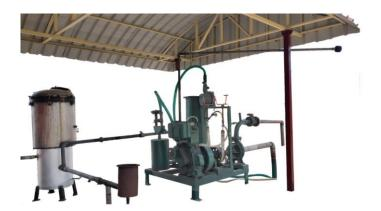
A downdraft gasifier along with a gas cleaning system retrofitted with a 5 Hp diesel engine coupled with a centrifugal pump for pumping water for irrigation applications. In
