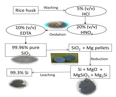
Production of high purity solar grade silicon from rice husk through magnesio thermic reduction process
