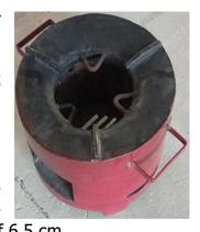
Rectangular opening of  $10\times 5$  cm is provided in the chula outer wall for the entry of secondary air. The temperature of air inside the air heating space is always 4 to 5 °C higher than the ambient air. The overall dimensions of metal Chula is 31 cm X 29 cm.
