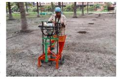
engine was relocated to the handle of the frame, so that the acceleration may be given to the auger bit simultaneously when the Auger unit is pressed down to form pits. The total weight of the unit was 44.5 kg.
