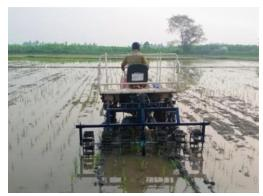
can be covered in a single pass of operation. The width of the rotary unit is 150 mm. The entire unit can be easily mounted and dismantled from the transplanter. Drive for the weeding unit is taken from the Power Take Off (PTO) of the transplanter. The gear box, rotary weeding drums and floats are mounted on a frame.
