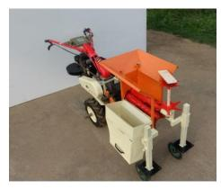
snapping rollers spin opposite to each other to grab the stalk just below the cob and guide them into the rolls, and the rotary cutting blade provided at the bottom cuts the maize stalk at ground level. The snapping rollers were fixed at different levels to collect the harvested cobs in the box provided by the side of the rollers.
