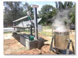
respectively. Substrate (2-5 cm size) of 120 kg/day (dry weight) with hot water pasteurization at temperature range of 70-80°C was observed.
