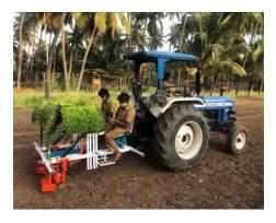
be resting at an angle of  $75^{\circ}$  so that entire tray height will be within the reach envelope zone. Both the hands can be used to pick the seedlings from the tray and placing it in the seedling conveyor
