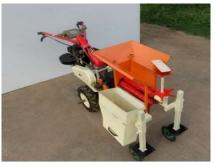
on their surfaces was adopted for shearing of cobs from the plants. The snapping rollers spin opposite to each other to grab the stalk just below the cob and guide them into the rolls, and the rotary cutting blade provided at the bottom cuts the maize stalk at ground level. The snapping rollers were fixed at different levels to collect the harvested cobs in the box provided by the side of the rollers.
