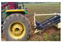
of 5300 mm, rotating in the opposite directions was used for conveying the dug plants from the blade to the stripping unit. The stripping system is having two rotating drums made of 4 rods provided with rubber flap of 650 x 60 mm to avoid the damage of pods. The length of the stripping rods was about 650 mm. The drums were rotating in the opposite directions. A box of 850 x 640 x 330 mm was mounted below the
