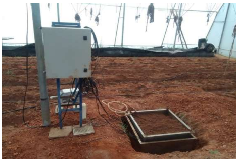
Digital lysimeter installed in the polyhouse
